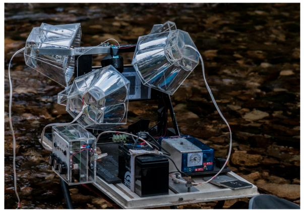
**FIGURE 18.** The experimental arrangement for testing the Vela One ultra high-speed flash system using three bulky early experimental reflector modules, each with 3 LEDs and associated reflectors. The electronic controller for the Vela One flash is mounted on the left side of the rig.
