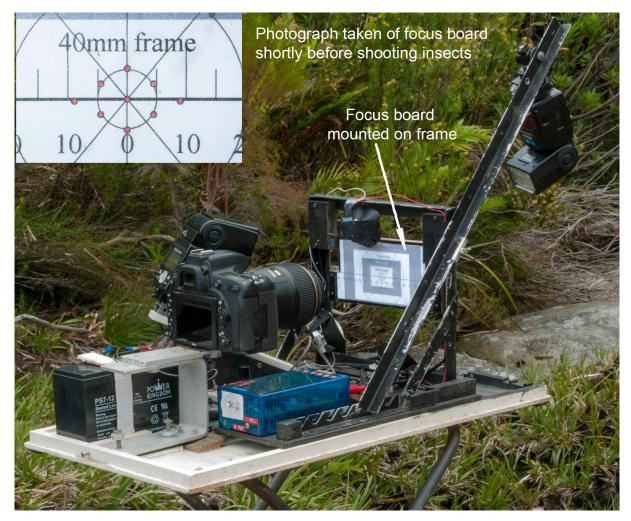
**FIGURE 4.** The assembled rig with focus board temporarily positioned on the frame for establishing camera settings. The inset image (top left) shows scale markings in mm and nine red dots indicating IR beam intersection points.
