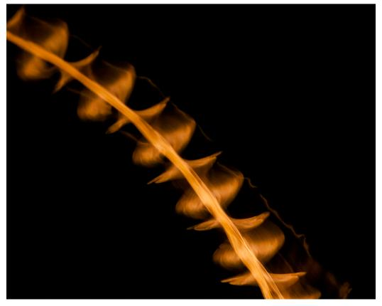
**FIGURE 10.** An insect flight trace using incandescent light only. The broad portions of the trace are created during the insect's downstroke. The upstrokes are narrow peaks between the downstrokes. Note orange colour of trace caused by reduced voltage from power drain on battery.
