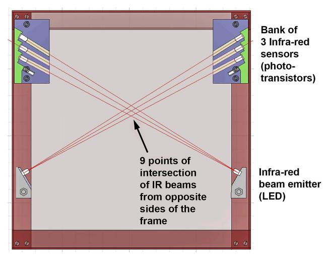
**FIGURE 3.** Diagram illustrating the frame and light beams arrangement. The camera is focussed on the plane which passes through the 9 points where the light beams intersect near the centre of the frame.
