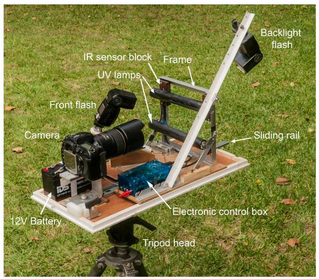
FIGURE 1. The assembled base of the rig with fixed electronic components and connected camera and speedlight flash units ready for use.
