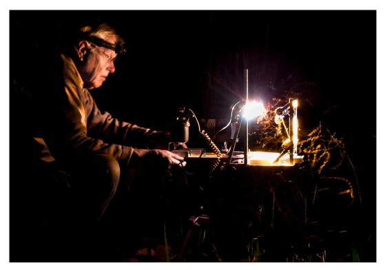
**FIGURE 9.** One of the authors operating an older form of the rig beside a river at night. Note the insects, here mainly *Athripsodes bergensis* Scott 1958, and their flight trails in the vicinity of the rig. The insects in this image are revealed by the electronic flash units. The orange trails are revealed by light from an incandescent supplementary lamp.
