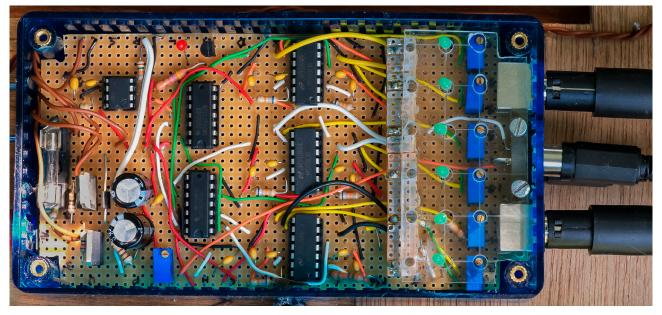
FIGURE 8. Top view of electronics control unit with the lid removed. Note the six green LED lights that glow when a beam is broken.
