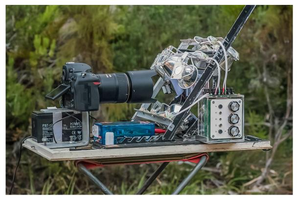
**FIGURE 19.** Later, more compact design of Vela One flash system, with nine individual smaller reflectors placed to align accurately with targeted picture frame. Note the electronic controller mounted on the right side of the rig.
