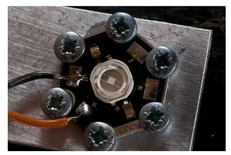
FIGURE 5. Ultraviolet LED used to attract insects to the general location of the frame.
