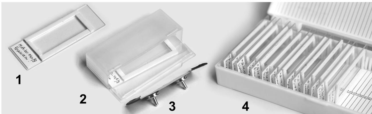
**FIGURES 1–4.** Silk samplers, boxes and specimen holder. 1, Silk sampler; 2, Small portable specimen box; 3, Specimen holder for SEM examination; 4, Slide box with silk samplers, for long-term storage.
